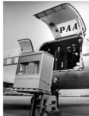
FIGURE 4.1: The IBM 305 RAMAC introduced in 1956 and weighing 1 Ton could hold 5 MB for the monthly price of $30,000.
